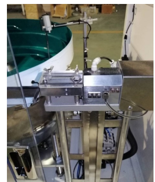
5mm Mini & 8mm Barbed Channel Lock Vibrator with Auto-Rotating Fastener Feeder.
