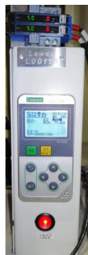
Vibrator and Automatic Magazine Fastener Feeder with a separate PLC controlled pendent for each feeder.
