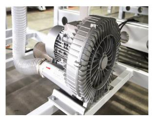
· The floating air receiving table with blower motor used for protection of finished parts.
