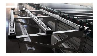
Extended out-feed table comes STANDARD allowing oversized parts to rotate back onto the receiving table.
