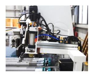
· Automatic adjustable small part diverter.
